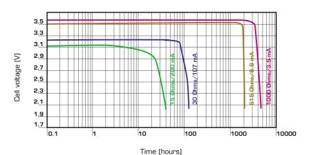
Typical discharge profiles at +20°C
