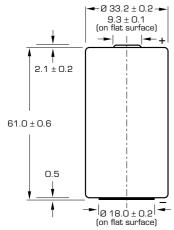
Finished version with protruding positive end cap
